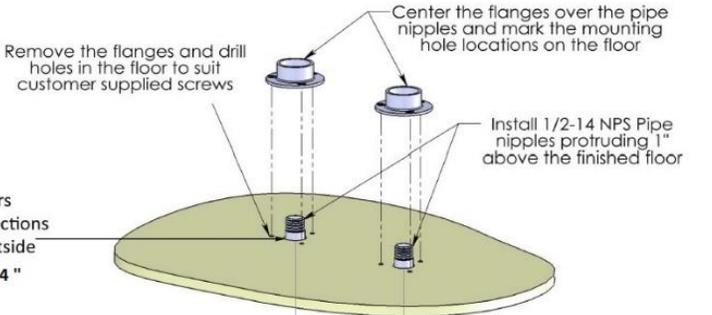
**Suggested Centers for Supply Connections from the Tub Outside Edge - 3" to 4"**
